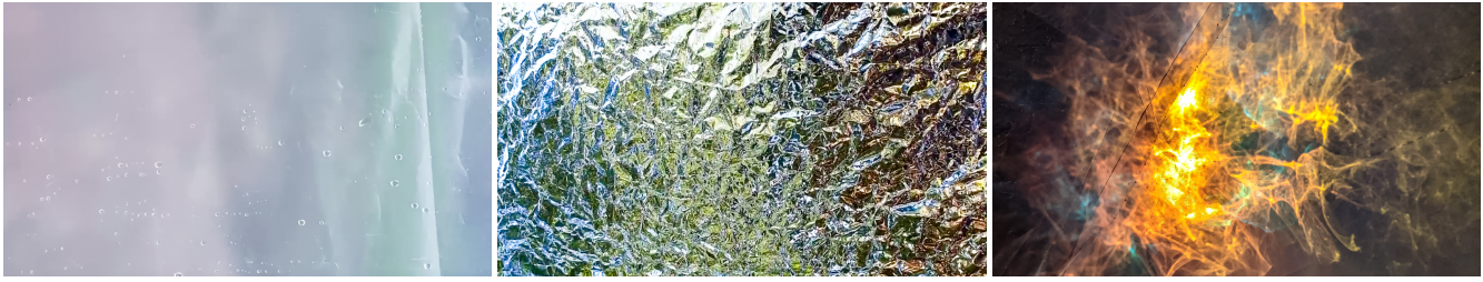
Figure 4: Textures: (left) Rain drops and wrinkles add textural memories of recent rainfalls and un/foldings. We used translucent polyethylene sheets (6mil thickness) because it is recyclable and durable. It diffuses light and blurs what is on the other side. (middle) The foil crinkles noisily. It both reflects light like a broken mirror and is slightly translucent. (right) Dichroic film splits light into multiple colors, shown here reflecting off of polyethylene around sunset.
